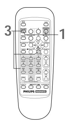
Point the remote control at your Cable Box/DBS. Press the CBL/DBS button, then press the POWER button. If your Cable Box/DBS turns on or off, try the CH(annel)  $\blacktriangle$  buttons. If the remote control operates the Cable Box/DBS, you're finished. If your Cable Box/DBS does not turn on or off, or if the CH(annel)  $\bigstar$  buttons don't work, go to step 2.
